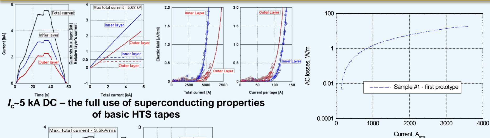
$I_c \sim 5 \text{ kA DC}$  – the full use of superconducting properties of basic HTS tapes
