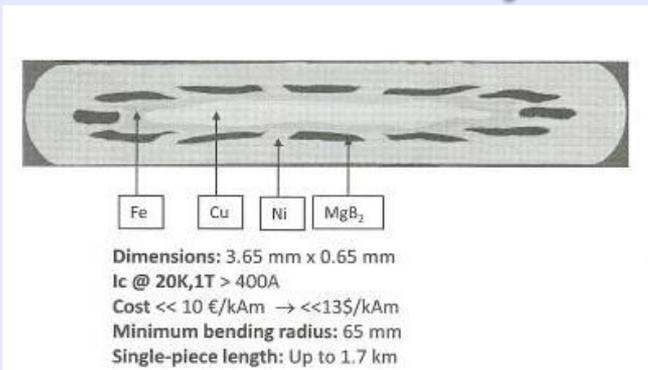
Basic tape: 3.65mm x 0.65 mm MgB<sub>2</sub>, Fe barrier, Ni matrix, Cu stabilizer
