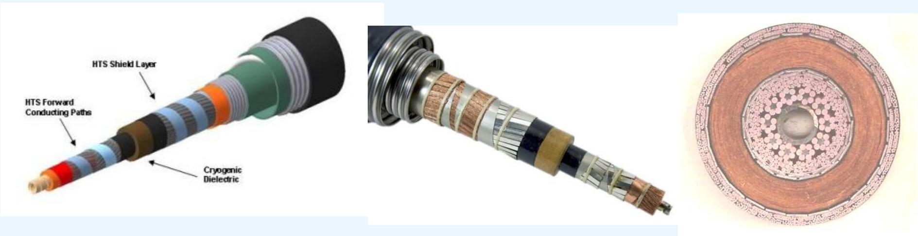
**200 m cable design is quite similar to those of 30 m cable. Only superconducting shield made sufficient difference from 30 m cable design**
