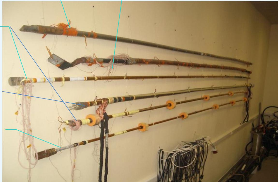
**In total 8+ models of 5-m cables have been tested up to now including first cable model with Russian 2G wire produced by SupeOx company**
