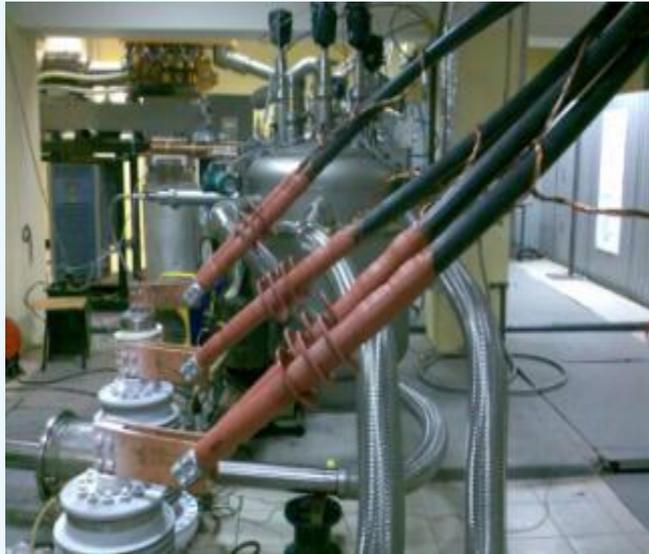
Current leads connected to cryostats in a cryogenic system.
