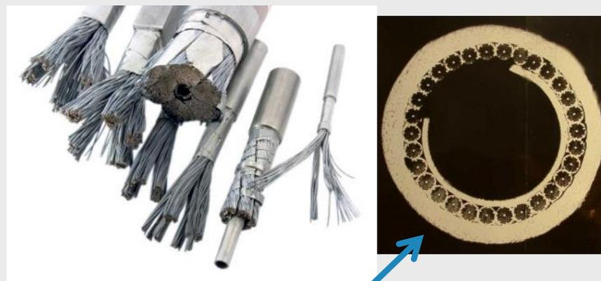
The most miniature CICC in the world: outer diameter – 6.4 mm; 30 NbTi strands 0.5 mm each. Developed by VNIIEP for SIS-100 project in GSI Darmstadt.
