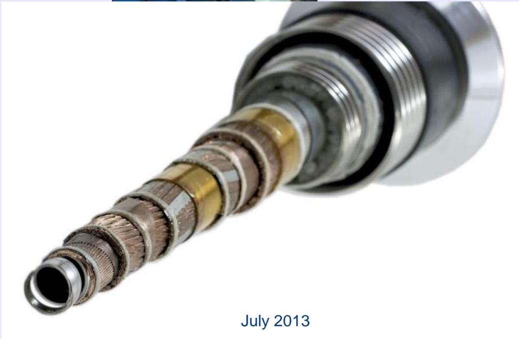
The cable has been made with standard cable equipment with technologies similar to those used for HTS cables.
