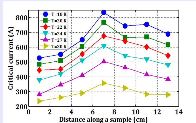
$I_c$  non-uniformity has been observed but results in wires are better than specifications from Columbus Superconductor.
