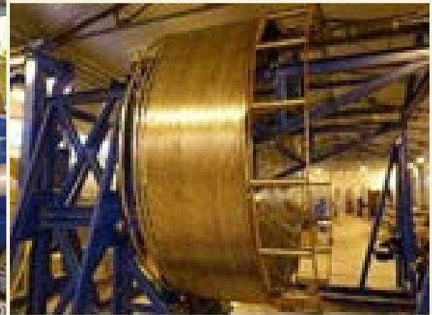
Trial conductor on the winder
