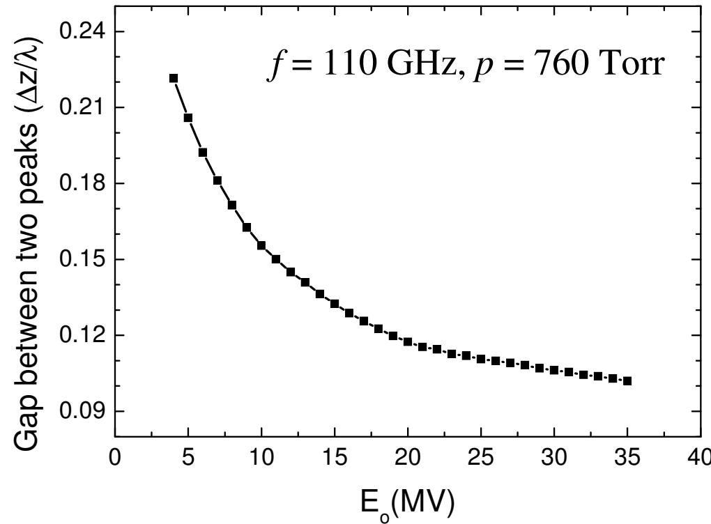
Increasing field strength decreases filament spacing as breakdown threshold is exceeded closer to the previous filament.
