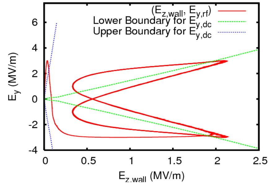
high field susceptibility becomes vertical in waveguide – no upper field cutoff
