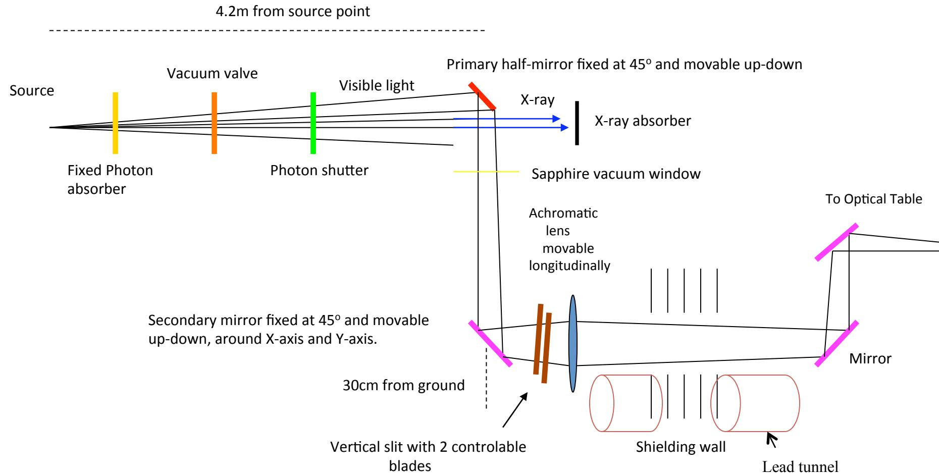
Total beamline length = 2 [4.2m (source-1<sup>st</sup> mirror) + 1.1m (1<sup>st</sup>-2<sup>nd</sup> mirror)+0.4m (1<sup>st</sup> mirror-lens)] =11.4 m.
