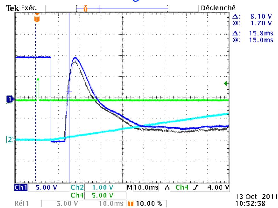
As for the tracking QF vs Dipole, once the offset is tuned on the quadrupole power Supply, the tracking error measurement ( $\pm 2.10^{-3}$ ) remains very stable while the power supplies are running.
