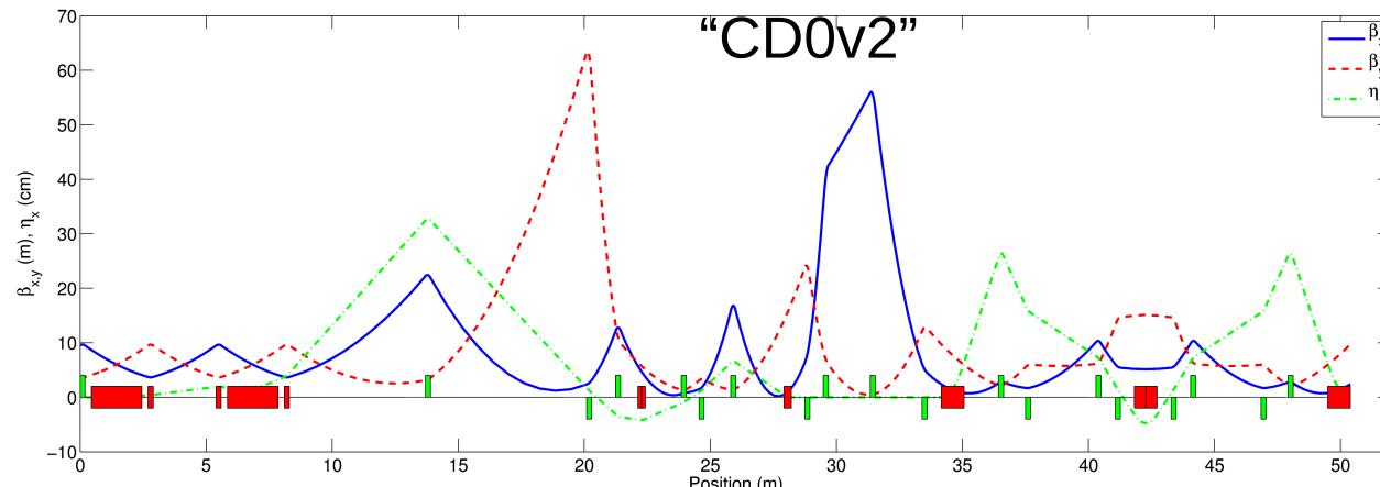
The new design (CD0v2) has the same performance to the original design in terms of CSR effects, magnet tolerance and high order chromatic effects.
