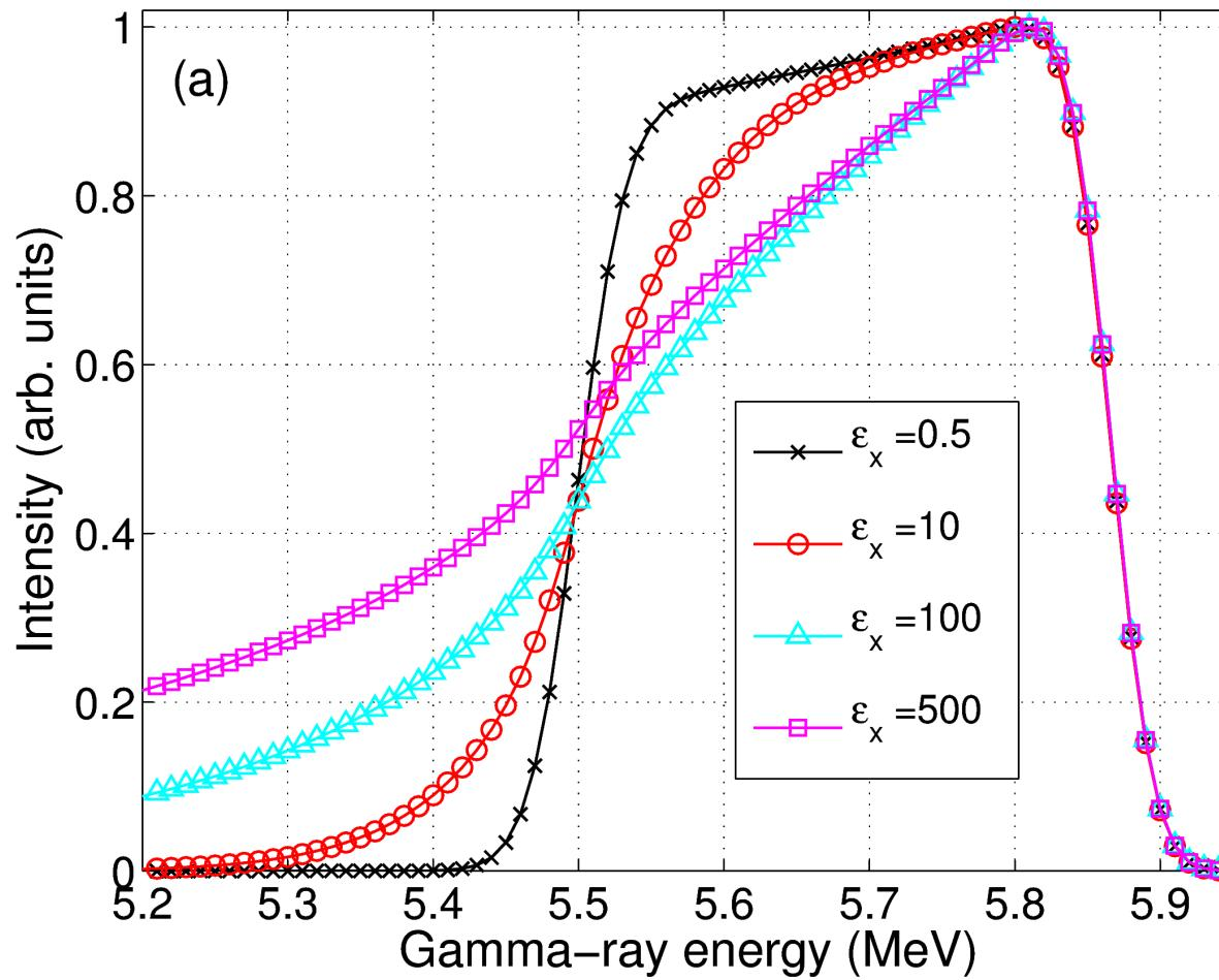
The electron beam emittance has no impact on the high energy edge of the spectrum if the collimation aperture is large enough.
