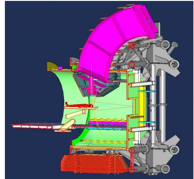
HIT 90 degree bend weigh 90 tons, 65% of total gantry weight
