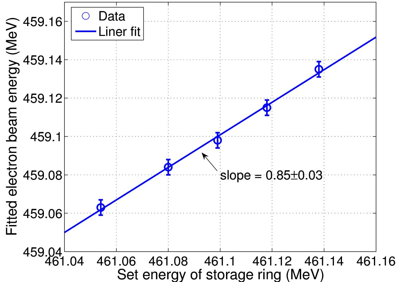
TAB. 1 – Uncertainty of the electron beam energy measurement at the storage ring set-energy of 461.06 MeV.
