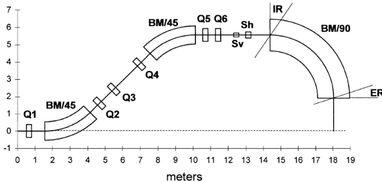
Fig. 3. Layout of the gantry with the minimum number of quadrupoles: Q1–Q6 = quadrupoles, BM/45 =  $45^\circ$  bending magnet, BM/90 =  $90^\circ$  bending magnet, Sh = horizontal scanner, Sv = vertical scanner, IR = input pole face rotation ( $30^\circ$ ), ER = exit pole face rotation ( $21^\circ$ ).
