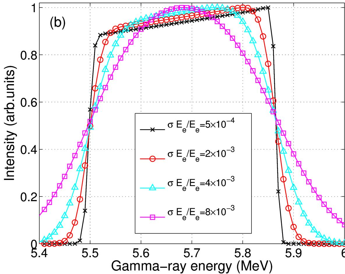
500 MeV electron beam scattering with 800 nm laser beam, and the radius of the collimation aperture is 16mm
