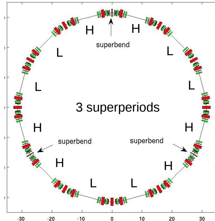
*Genetic Algorithm (GA) is used to design these high-low beta lattices*
