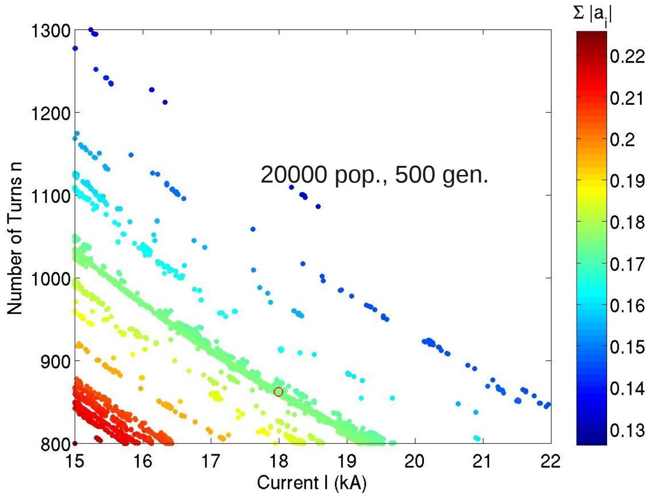
Trade-off between current  $I$ , winding turns  $n$ , and coefficient  $a_i$ :
