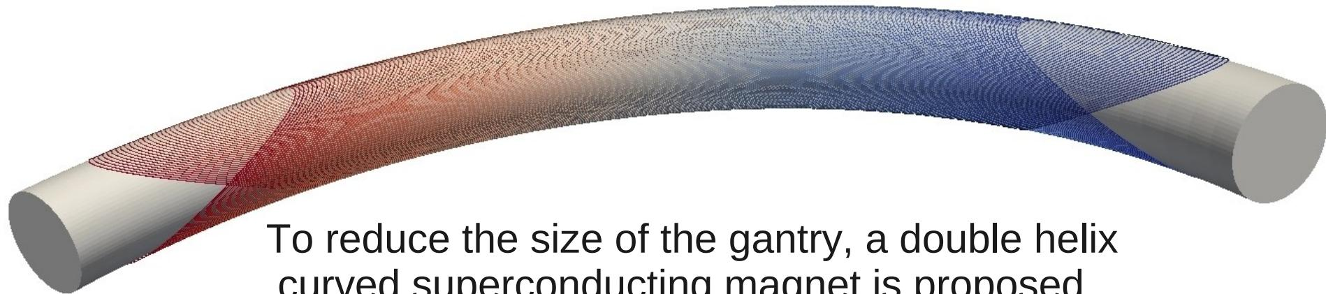
To reduce the size of the gantry, a double helix curved superconducting magnet is proposed.
