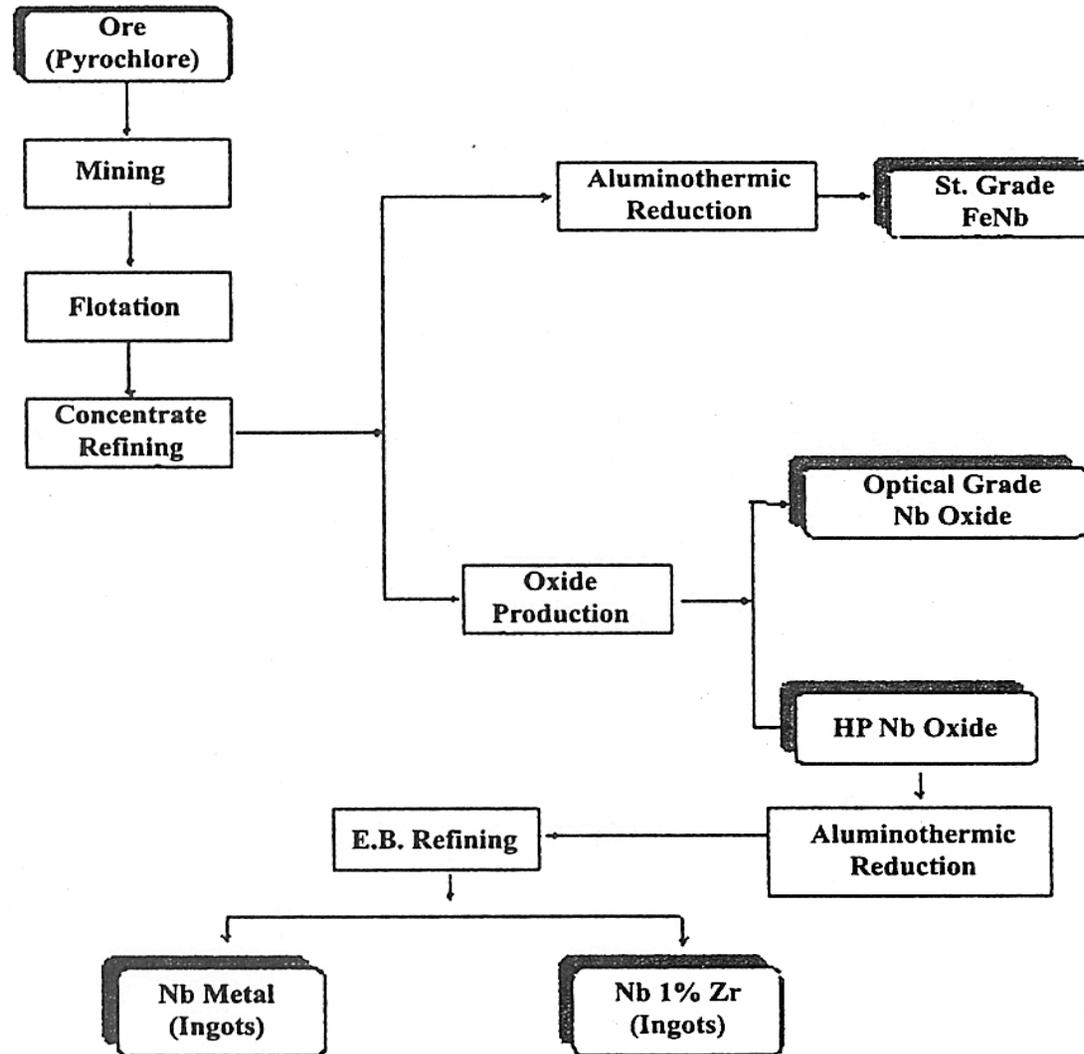
Fig. 3: Production flow chart at CBMM.
