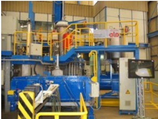
Electron beam furnace for the refinement of Niobium metal, producing 210 tons per annum
