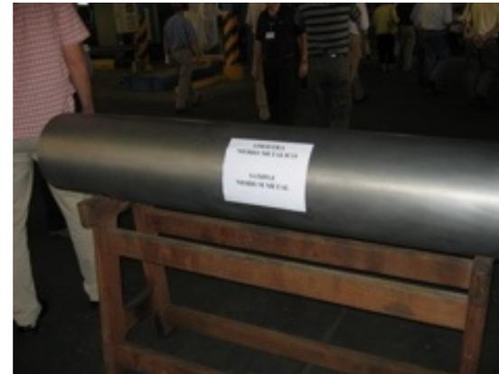
Finished Nb ingot from the Pyrochlore ore
