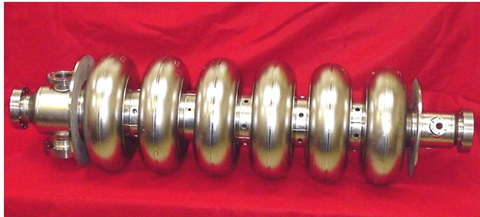
**~90% of CEBAF cavities were made with CBMM Pyrochlore ore based niobium
