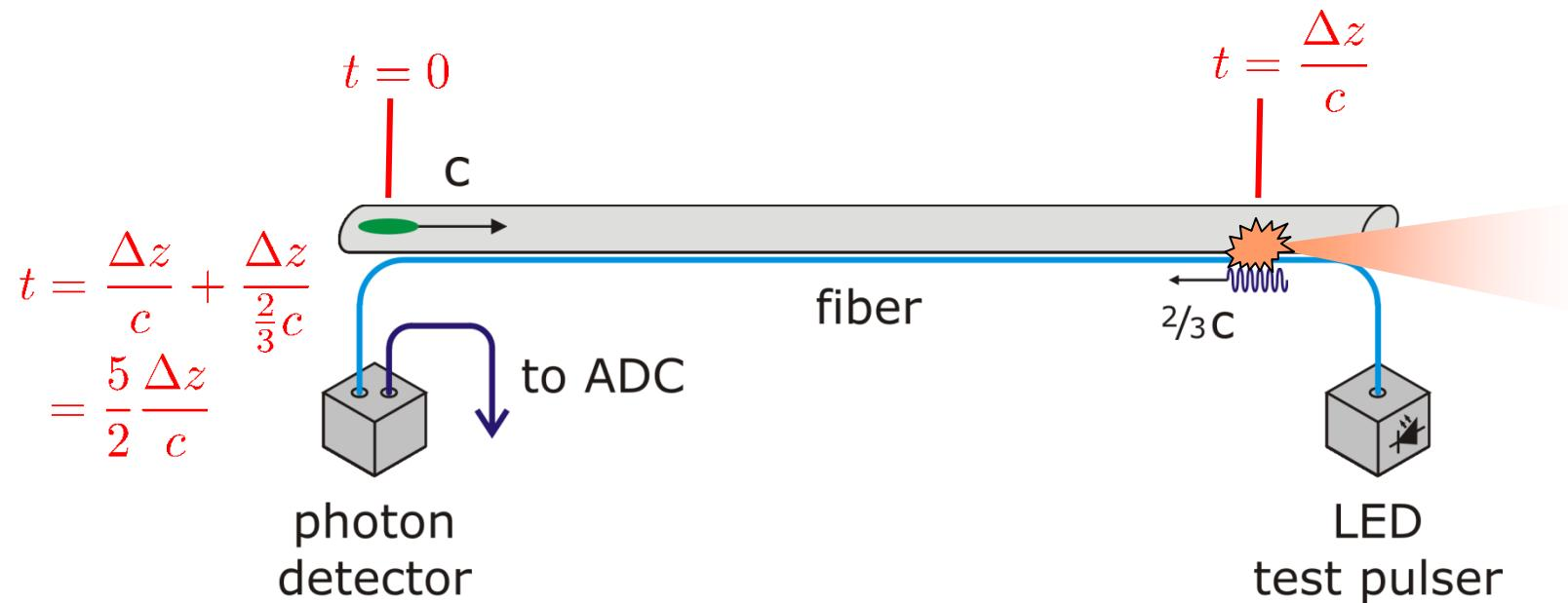
250 MS/s ADC → longitudinal resolution ~50 cm
