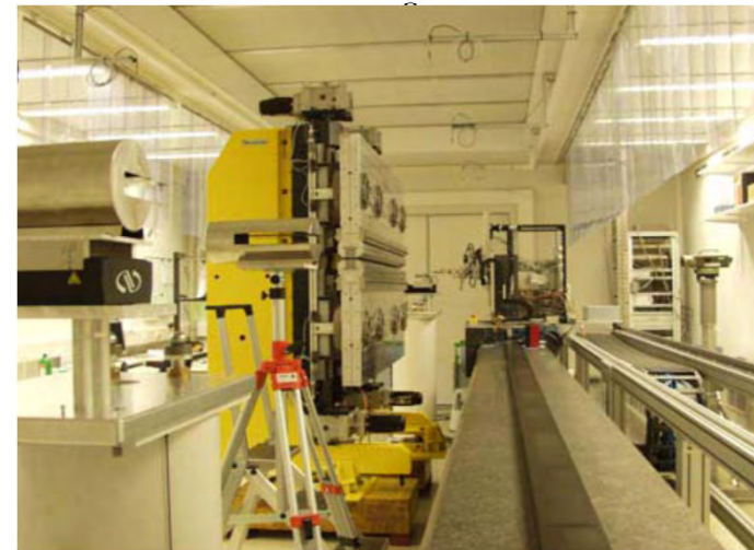
PETRA III undulator (XFEL prototype) in XFEL undulator measurement lab
